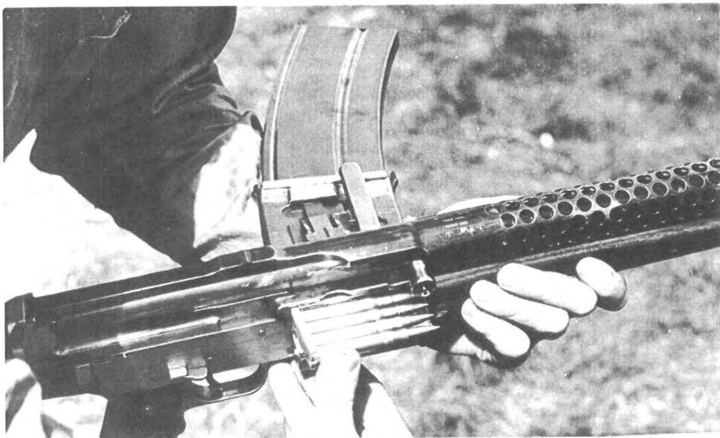
The M1941 LMG could be "topped off" using M1903 rifle five-round stripper clips. Image: Author's collection
