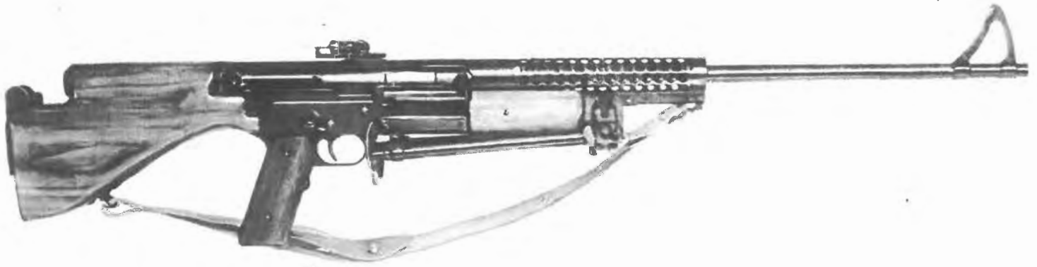
The M1941 Johnson LMG featured a straight-line stock with an exceptionally tall front sight. Image: Author's collection
