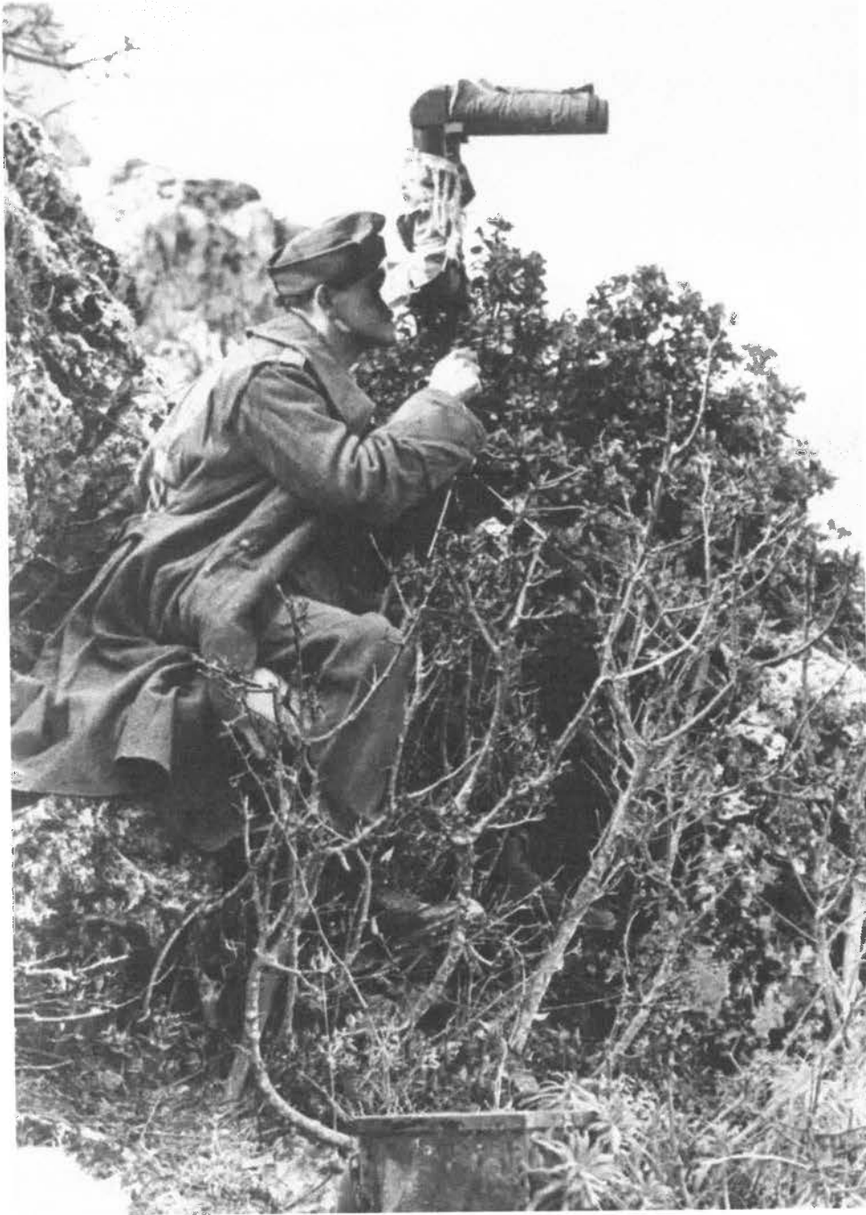
A German observer uses Scherenfernrohr SF14ZGi scissor binoculars, equipped with sun visors and camouflaged with fabric, during the Battle of Monte Cassino. Image: Polish National Digital Archives
